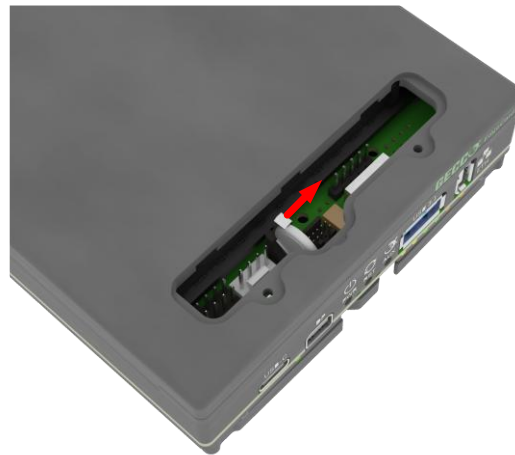
Figure 3. EdgeCard RTC battery replacement
