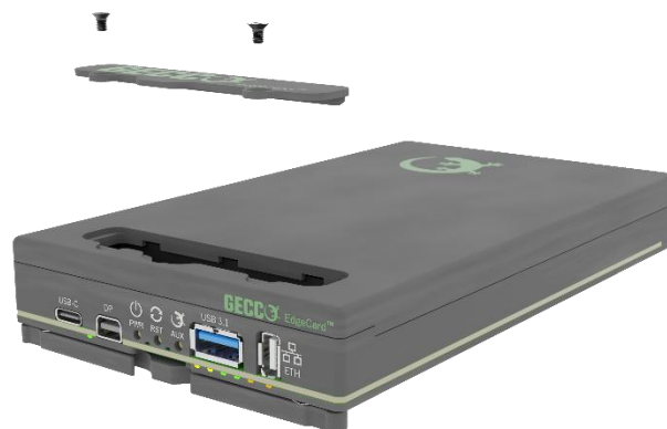
Figure 2. Access to RTC battery on the EdgeCard Server.
