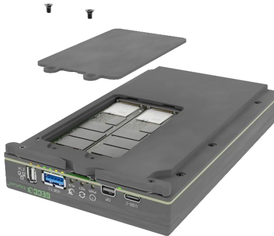
Figure 1. Access to M.2 Expansion Slots
