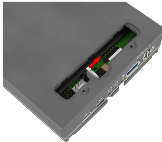
Figure 3. EdgeCard RTC battery replacement
