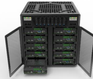
Figure 3. Compact VPX-aligned computing pod in a 10-inch cube chassis
